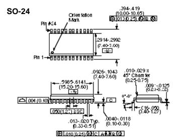
24-Lead SOP putting dimensions Wide body 300 (Au aimensions per u⊫u ∋o no. 1765-1715-170, issue oj Dimensions in ( ) are in mm.
