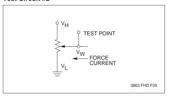
**Notes:** (1) Absolute Linearity is utilized to determine actual wiper voltage versus expected voltage =  $(V_{w(n)}(actual) - V_{w(n)}(expected)) = \pm 1$  MI Maximum.
