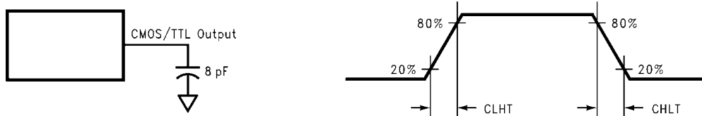
FIGURE 4. DS90CF386/DS90CF366 (Receiver) CMOS/TTL Output Load and Transition Times
